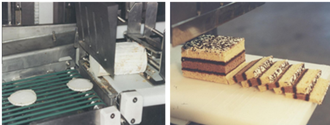
Fig. 4. Difference in cutting slices of a bakery product cut with and without ultrasound.
